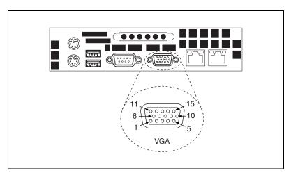
Figure 3-5. VGA Connector Location and Pinout
